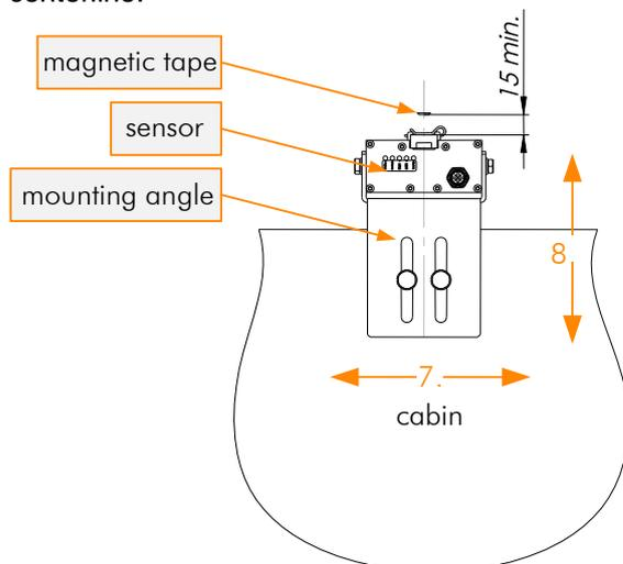
8. Adjust now the distance between sensor and band. Up to a travel height of 50m we recommend an offset of at least 15 mm. This will ensure steady contact between steel side of the band and the polymer guide of the sensor. In higher installations this distance may be increased.
