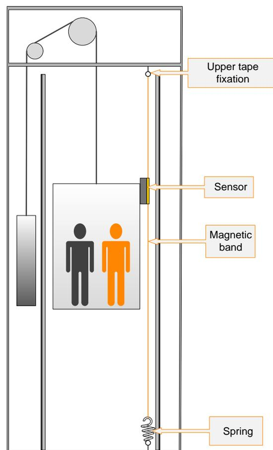
LIMAX02 can be installed at any position in the hoistway, depending on space situation and layout of the particular elevator installation.
