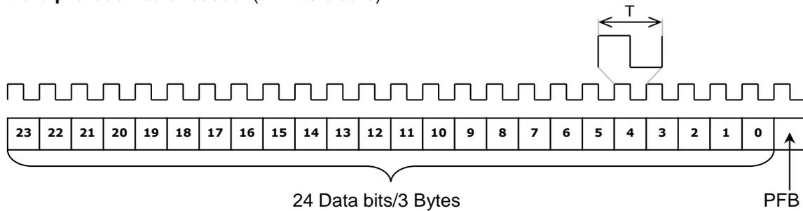
PFB = Power Failure Bit
