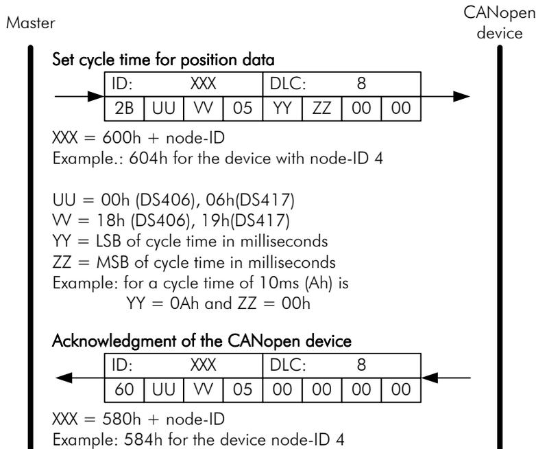
3. If the settings should be maintained in case of a power failure, the changes have to be saved, as described in section 7.4.5.
