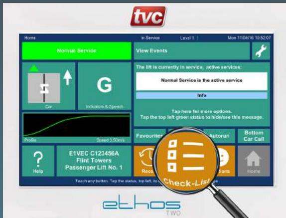
**Check List button** -this provides the lift engineer with simple step by step commissioning and testing functions, simply touch the relevant button to guide you through the process.
