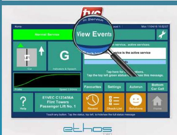
**View Events** - View the latest events which are colour coded from breakdowns, faults, service and general info. All events can be filtered and marked offering the engineer more control.
