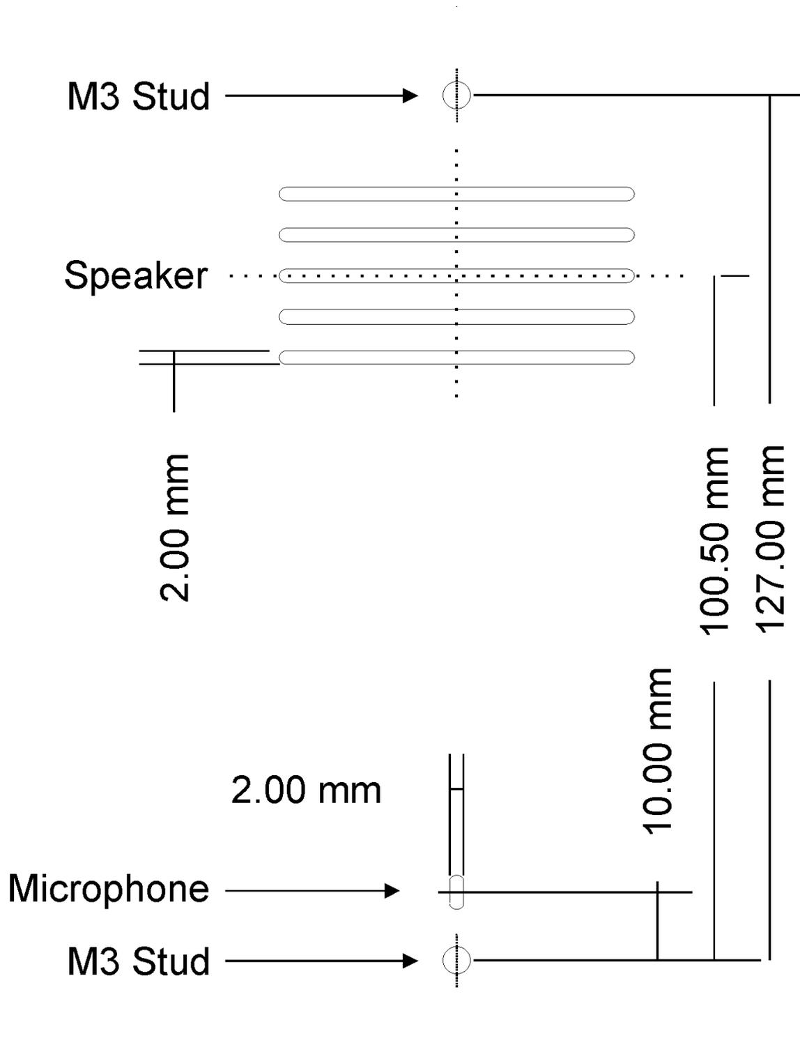
Figure 3- Stud Mounting & Grill Cut-out Positioning
