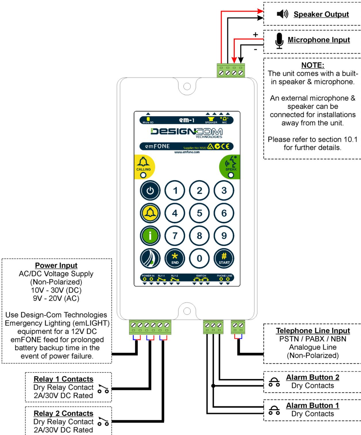
Figure 1- Wiring Diagram
