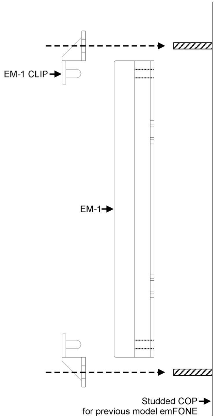
Figure 4 - Installation using Mounting Clips
