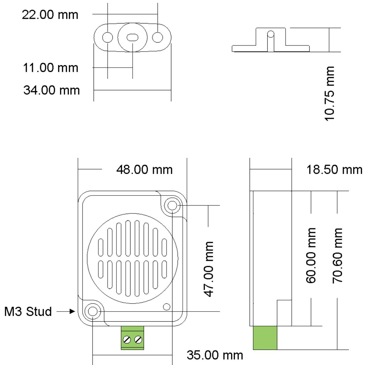
Figure 5 - External Microphone and Speaker Kit Stud Mounting and Dimensions
