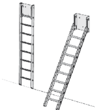
Ladder left: Vertical position Ladder right: Inclined position
